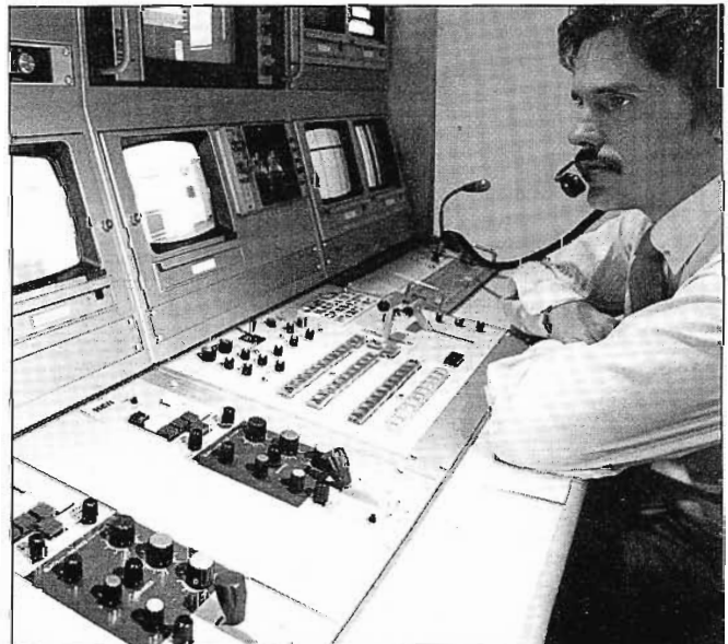
Producer/Director John Butler mans switcher in production control. Remote control units for TK-47 cameras are two panels in foreground.
